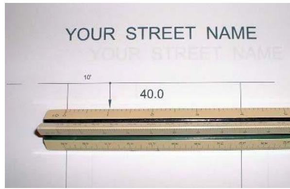
Fig. 3 Measuring 10 feet from the property line
