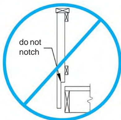
Figure34: Post Notches Prohibited
